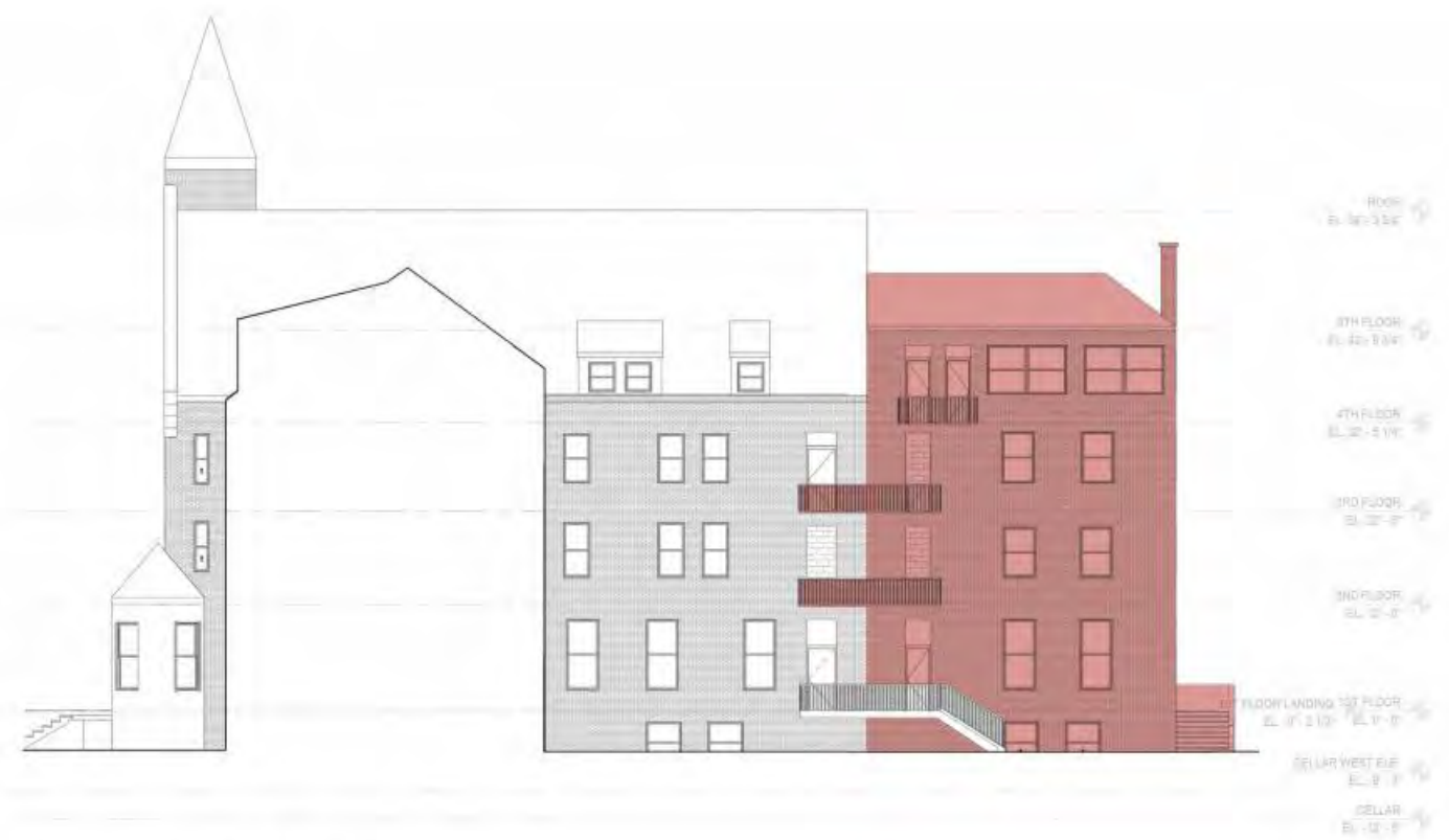
WEST SECTION REMOVAL
