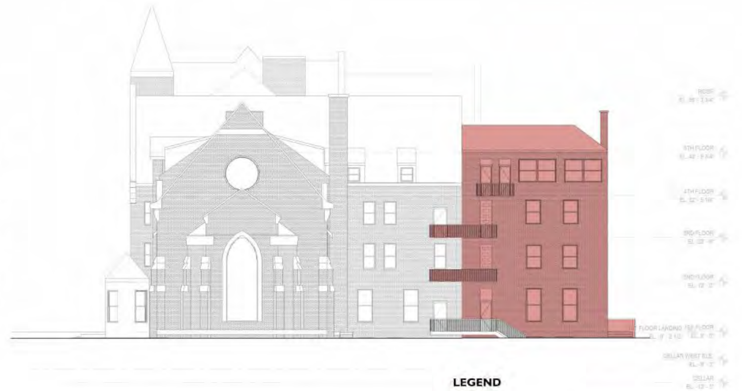
WEST ELEVATION REMOVAL
